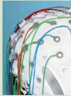
A skull cap with electrodes, used as a part of an EEG Experiment which involves measuring the electrical activity in the brain whilst a participant takes part in a task.
